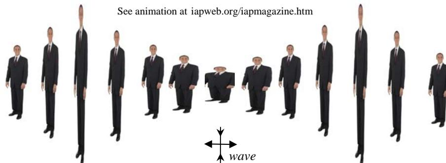
The gravity wave comes into the page, hits the man's stomach, and stretches and smashes him over time. The man starts his normal size on the left, and, as the gravity wave goes by, we see him change at various points in time. Note that the wave stretches everything so the earth is also stretched.
