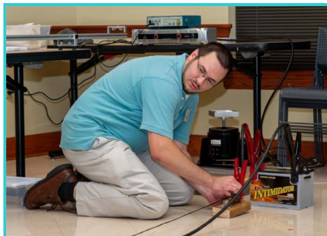
Ampere's force Law experiment: (top right and middle-left) Using a car battery, a switch, and jumper cables, the cables would attract or repel when nearly 800 Amps of current flowed through the circuit. The attraction and repulsion evidence that charge, when activated by impetus, can cause and receive a new field, the magnetic field.
